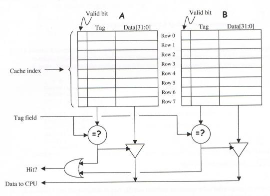
Each cache line holds a single 32-bit word of data along with its associated tag and valid bit (0 when the cache line is invalid, 1 when the cache line is valid).
