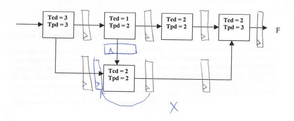
**4(b)** [3 points] Assume the same circuit (duplicated below) is pipelined for a throughput of 1/5 using the minimum number of registers. What is the latency?
