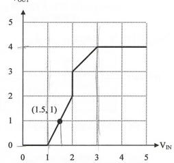
noise margins you can using these devices. Fill in your answers below, together with the resulting noise margins. You'll get partial credit for anything that works with nonzero noise margins; for all six points, maximize each of the noise margins. [Extra copies of these diagrams are attached to this test for scratch purposes].
