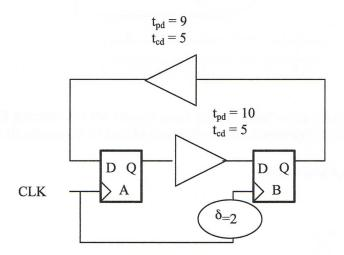
1(a). [3 points]: For the chosen clock period, what is the maximum setup time for the flip-flops for which the circuit functions correctly? As stated above, you can assume that the two flip-flops have identical setup times.
