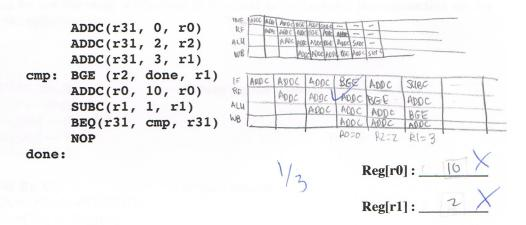
(C) [2 points]: Insert a minimum number of NOPs into the code below that will ensure that Adrian's 4-stage pipe produces the same values in r0 and r1 as the unpipelined processor.
