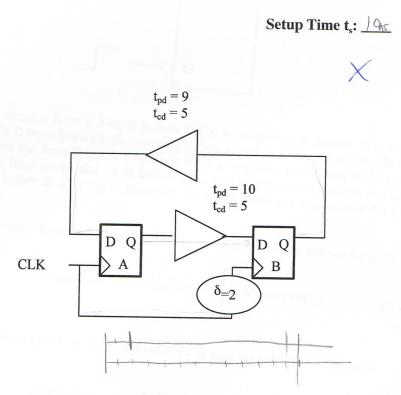
1(b). [3 points]: For the chosen clock period, what is the maximum hold time for the flip-flops for which the circuit functions correctly?
